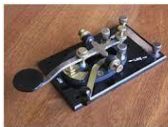
Telegraph key for sending Morse code by electricity
